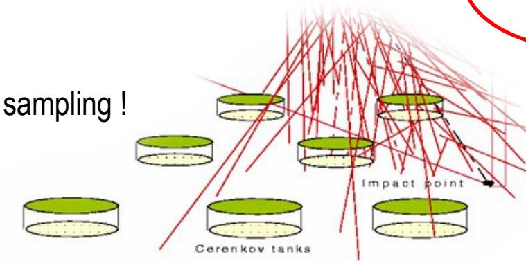
At high altitudes and/or energies also hadrons and  $e^-$ ,  $e^+$ ,  $\gamma$  can be measured
